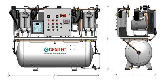
SHOWN: Duplex 5 HP reciprocating compressors mounted on a 120 gallon horizontal A.S.M.E. air receiver with desiccant dryers, filters, regulators, CO and dew point monitors. Includes duplex Nema 12 control panel. Package is NFPA99 compliant.
